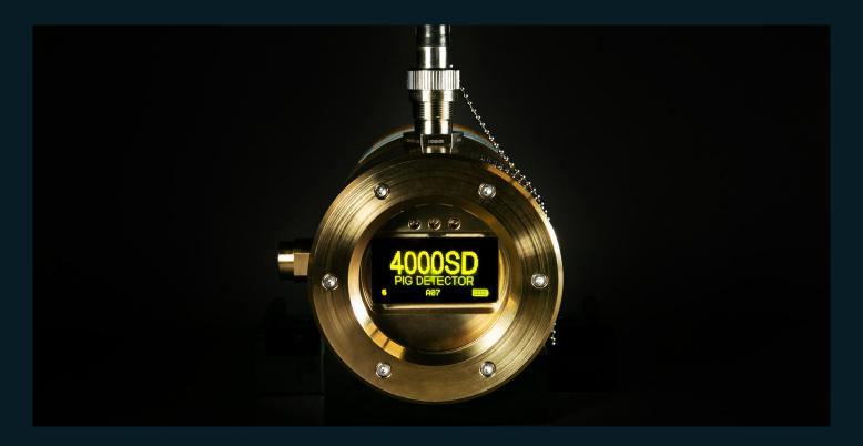
The 4000SD pig signaller is a compact, non-intrusive, magnetic signaller suitable for harsh subsea applications. The 4000SD detects, logs and signals (via the display and LEDs) the passage of magnetic pigs at critical points along a subsea pipeline.
