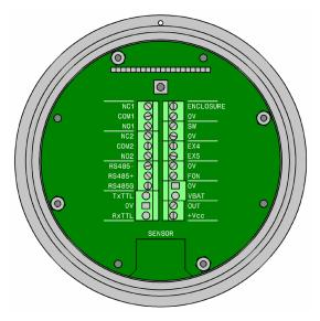
All connections are made using 5.08mm pitch removable terminal blocks which can accept up to 2.5mm<sup>2</sup> (14AWG) wire size. All connections must be made using suitable crimp ferrules. Connections are clearly labelled on the PCB and have the following functions:
