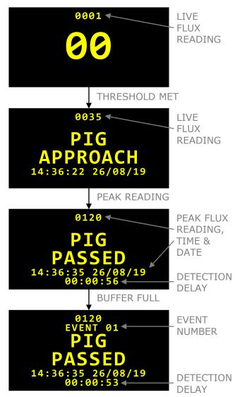
If PIG APPROACH is displayed but the pig stops near the signaller without causing a sufficient peak then the signaller shall return to LISTENING 3 minutes and 24 seconds after displaying PIG APPROACH without displaying PIG PASSED or starting the DETECTION DELAY. This will be logged as an event however no event will be signalled via the LEDs or any other interface such as relays or current loop.
