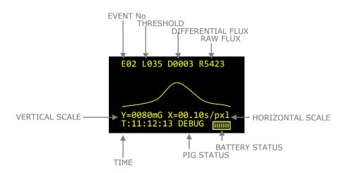
This setting can be very useful for determining the magnetic signature of a pig. However, this mode should never be used for regular pig signalling. See also 4.5.1 DEBUG MODE.
