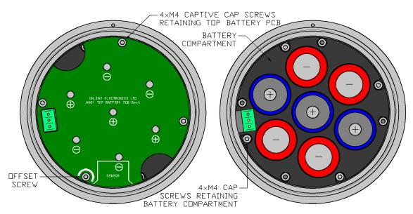
The unit will shut down when the battery voltage reaches 6.5V ALKALINE or 17.0V LITHIUM. To replace the batteries, follow the steps below:
