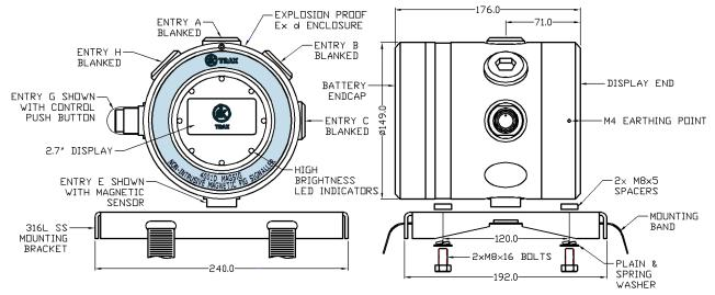
**REMOTE SENSOR OPTION:** The magnetic sensor can be supplied on a cable up to 10m long for use with buried pipelines or when access is limited. The protection concept for the remote sensor is intrinsically safe 'ia'.
