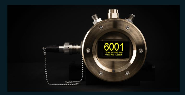
The 6001SD Temperature and Pressure Subsea Logger is a compact, self-contained, subsea unit which logs and displays readings from internal digital pressure and temperature sensors. The 6001SD can confirm a successful hydrotest without needing to recover the unit. An extended housing version enables longer battery life as well as the capability to utilise a Luma Optical Modem.
