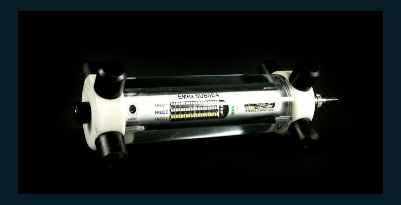
The EMRx Subsea Receiver is a robust, state of the art, multi-frequency, electromagnetic (EM) receiver used for locating lost or stalled pigs and tracking pigs fitted with any EM pig transmitters or magnets. It can also be used to confirm a pig has left or arrived at a particular location and for general monitoring of pig movements.
