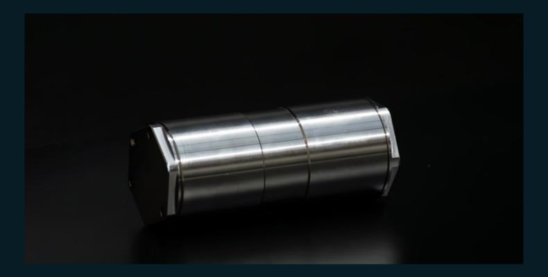
The EMTx20 transmitter is an electromagnetic (EM) transmitter that can be used for pig tracking and locating functions, intended for use in pipeline diameters above 4" to 8". The transmitters operate effectively in every type of pipeline, i.e. topside, buried, gas or liquid and in pipeline bundles where acoustic transmitters are either less effective or ineffective.
