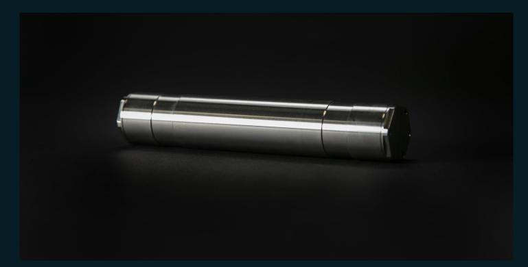
The EMTx20 transmitter is an ATEX certified electromagnetic (EM) transmitter that can be used for pig tracking and locating functions, intended for use in pipeline diameters above 4" to 8". The transmitters operate effectively in every type of pipeline, i.e. topside, buried, gas or liquid and in pipeline bundles where acoustic transmitters are either less effective or ineffective.
