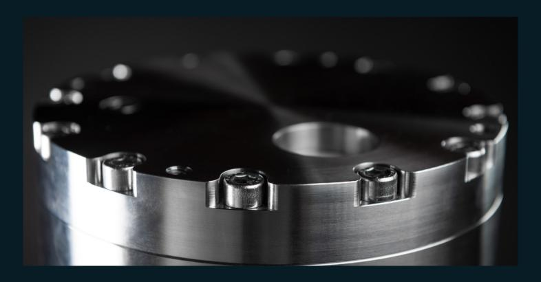
The EMTx50 HP transmitter is a high-pressure electromagnetic (EM) transmitter that can be used for pig tracking and locating functions, intended for use in pipeline diameters of around 16" and above. The transmitters operate effectively in every type of pipeline, i.e. topside, buried, gas or liquid and in pipeline bundles where acoustic transmitters are either less effective or ineffective.
