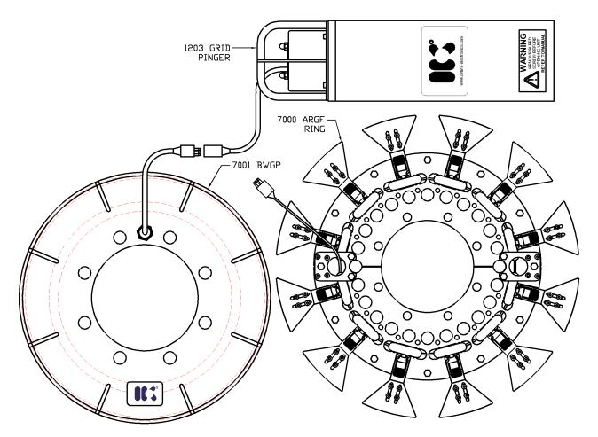
The current system can be manufactured to specific project specifications and supplied with a GRID<sup>®</sup> Pinger. The 7000 ARGF Ring is typically suitable for 10" pipelines or larger.
