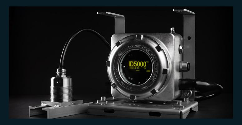
The ID5000 (Active) is a fully ATEX certified, non-intrusive pig signaller which detects, signals and logs the passage of pigs at critical points along a liquid pipeline both onshore and offshore. The ID5000A can also be used to confirm the position of pigs in the receiver.
