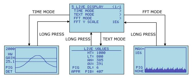
**TIME MODE** – This mode displays a live graphical plot of the Difference Level (DL) vs time. The High Threshold (HT) and the Low Threshold (LT) are indicated by the dashed lines. The Y axis is auto scaling based on the maximum value of Difference Level (DL).
