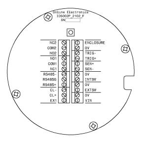
An example of the recommended wiring for an ID5002P system is shown below.
