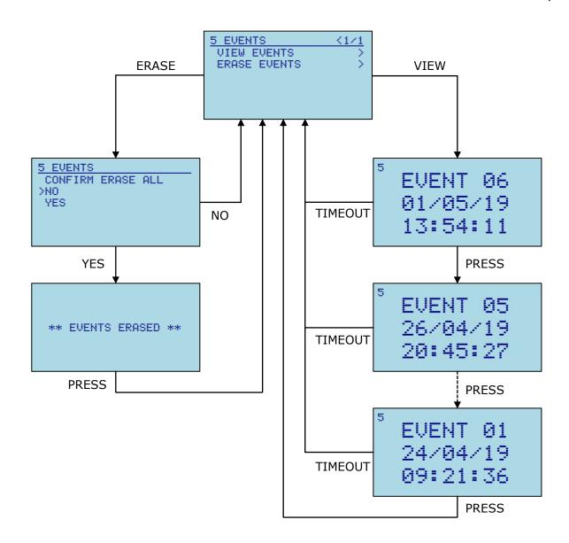
**VIEW EVENTS** – Selecting this item will allow the user to cycle through all logged EVENTS from newest to oldest. The EVENT number, date and time are shown. Pressing the CONTROL BUTTON will cycle to the next event. The CONTROL BUTTON can be held to pause at any event. If the COUNTDOWN INDICATOR reaches 0 then the unit will return to the EVENTS MENU.
