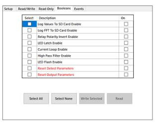
press the WRITE SELECTED button. If the write is successful a message will be displayed in the status bar located in the bottom left corner of the application window.
