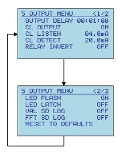
**CL DETECT** – Select this item to edit the CURRENT LOOP DETECTION level (4.0 – 20.0mA).
