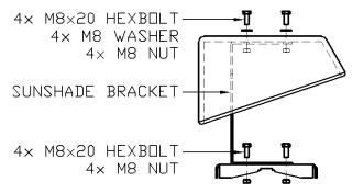
Secure 2x pipeline mount sunshade brackets to the mounting plate using 4x M8x20 hexbolts / 2x 'C' brackets / mounting plate / 4x M8 nuts.
