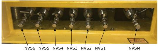
Note NVSn order counts from right to left Figure 3 Needle valve cover access
