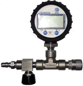
Figure 7 Charge manifold
