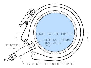
the sensor must be fitted on the lower half of the pipeline as shown to minimise convection heating.
