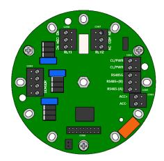
All connections are made using 5.0mm pitch pluggable terminal blocks which can accept up to 2.5mm2 (12AWG) wire size. All connections must be made using suitable crimp ferrules.
