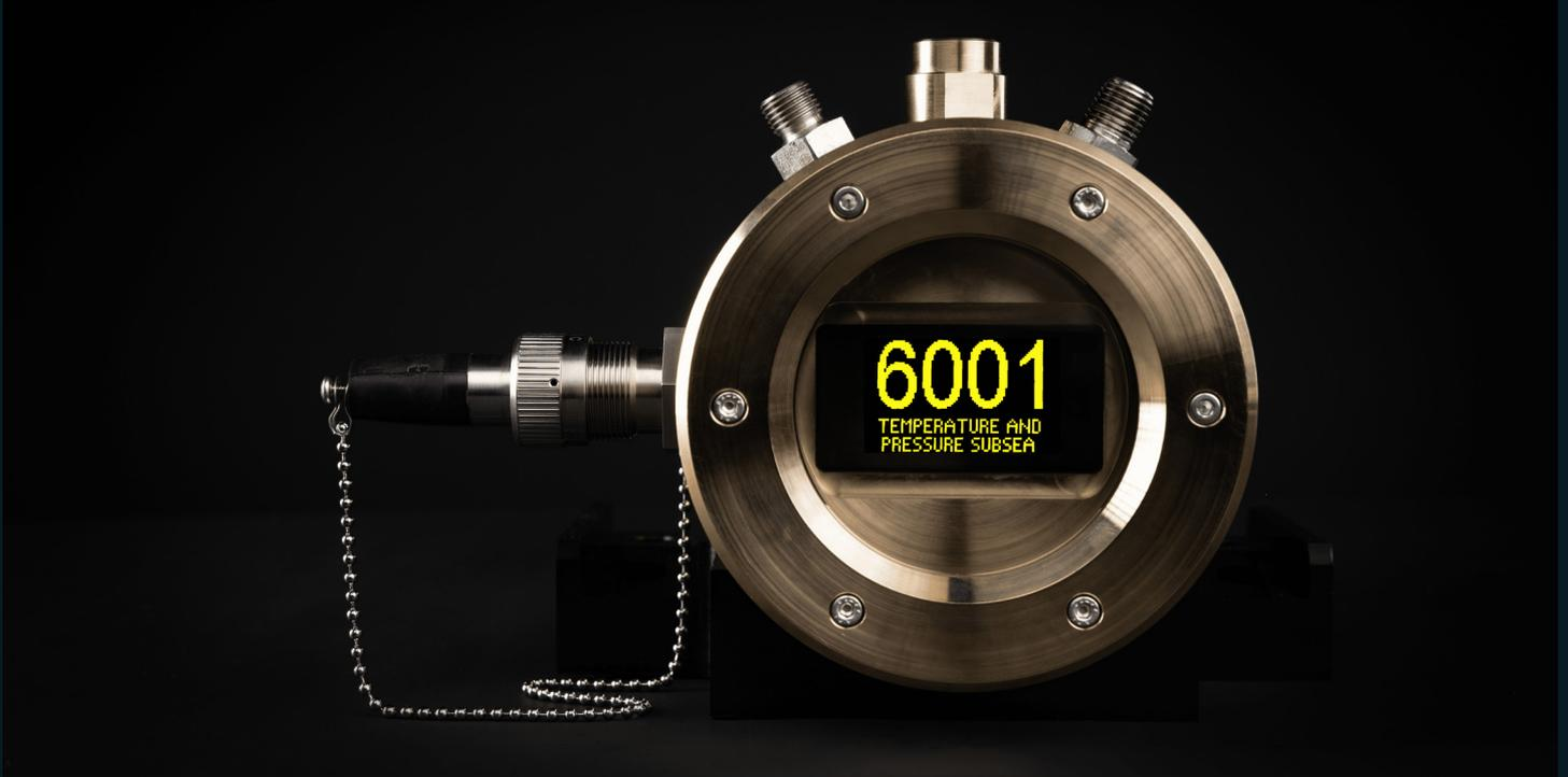
The 6001SD Temperature and Pressure Subsea Logger is a compact, self-contained, subsea unit which logs and displays readings from internal digital pressure and temperature sensors. The 6001SD can confirm a successful hydrotest without needing to recover the unit. An extended housing version enables longer battery life as well as the capability to utilise a Luma Optical Modem.
