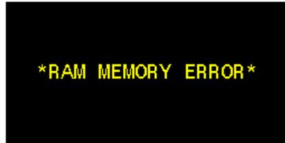
At switch ON the 6001SD conducts a self-check on the RTC circuitry as per section 4.1 TURNING ON. If any problems are found then the error message shown will be displayed and the 6001SD will reset all system variables to default values. Please contact Online Electronics Ltd if you see this message. The most likely cause is that the coin cell has expired. See section 12.3, ROUTINE MAINTENANCE AND STORAGE, for more information.
