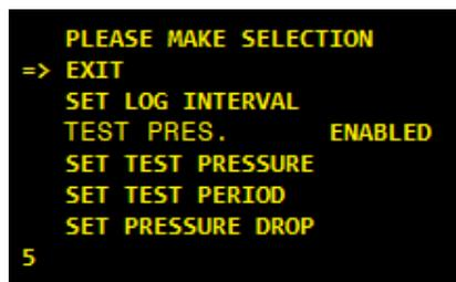
The PRESSURE TEST FUNCTION, when enabled, examines the data logged data for both pressure sensors obtained in the last TEST PERIOD hours of logged data. TEST PERIOD can be set from 1 to 60 hours.
