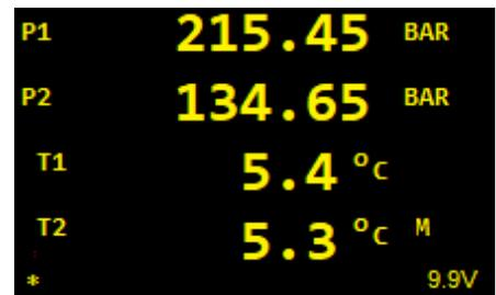
The current battery voltage is displayed at the bottom right of this screen. The battery packs should be changed if the voltage indicated is near 8V.
