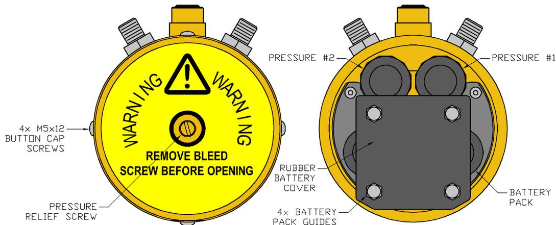
1. Opening of the unit should only take place in a clean, dry, laboratory environment.
