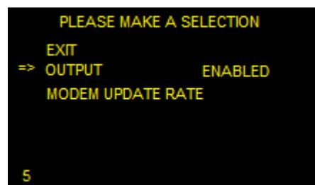
Selecting MODEM UPDATE RATE allows the selection of a pre-configured list of update times at which data is output to a connected OEL pinger. Selecting 0 minutes disables the transmission of data to a OEL pinger.
