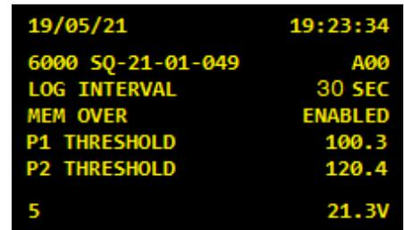
The unit then interrogates the sensors attached and displays their details. It also reads the temperature compensation from the sensors.
