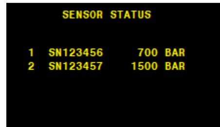
After displaying these screens the 6001SD will begin taking and displaying reading(s) from all enabled sensor(s). If the unit is configured for 30 second, 1, 2 or 5 minutes the display will show a LOG message to confirm logging at the configured LOG INTERVAL. No logging message is displayed for 1 second interval logging.
