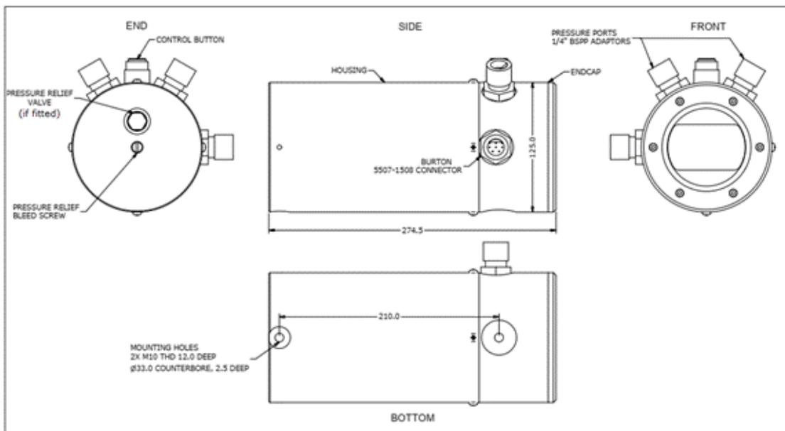
**MOUNTING OPTIONS:** As standard, the unit is supplied with 2x 12mm deep, M10 threads, 271 mm apart as shown above.
