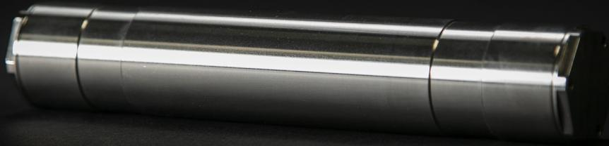
The EMTx20 transmitter is an ATEX certified electromagnetic (EM) transmitter that can be used for pig tracking and locating functions, intended for use in pipeline diameters above 4" to 8". The transmitters operate effectively in every type of pipeline, i.e. topside, buried, gas or liquid and in pipeline bundles where acoustic transmitters are either less effective or ineffective.
