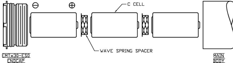
7. Once all cells are installed ensure that it is the FLAT, NEGATIVE END of the cells which you see when looking into the open end of the transmitter.
