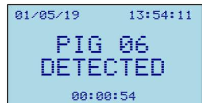
The unit will remain in the DETECTION state for the length of time defined by the OUTPUT DELAY before returning to LISTENING mode. The OUTPUT DELAY can be bypassed by pressing the CONTROL BUTTON.
