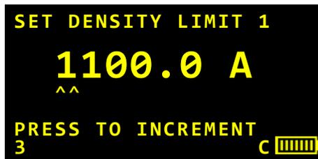
Figure 14 Setting density limit sub-menu
