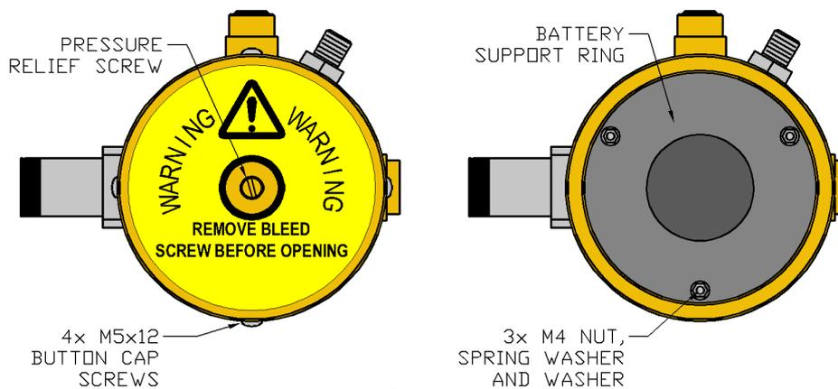
Figure 18 MEG ARTS® Controller Battery Removal
