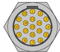
Figure 17 - CRE Size B Bulkhead Connector
