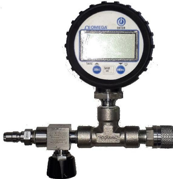
Figure 7 Charge manifold
