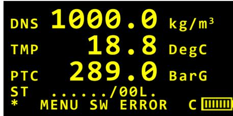
Figure 10 Default Screen showing MENU SW ERROR
