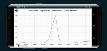
The IK Trax 4003 Pig Signaller App provides real-time alerts of any pig passage events, delivering detailed information directly to your device. It also allows you to easily update the parameters on the signaller. Available for Android, the app connects via Bluetooth for seamless operation.
