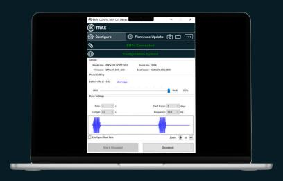
The IK Trax EMTx Config Android App provides an intuitive interface for configuring the EMTx series of EM transmitters. Available for both Android and Windows, the app allows users to connect via Bluetooth or a USB endcap (transmitter model dependent.)
