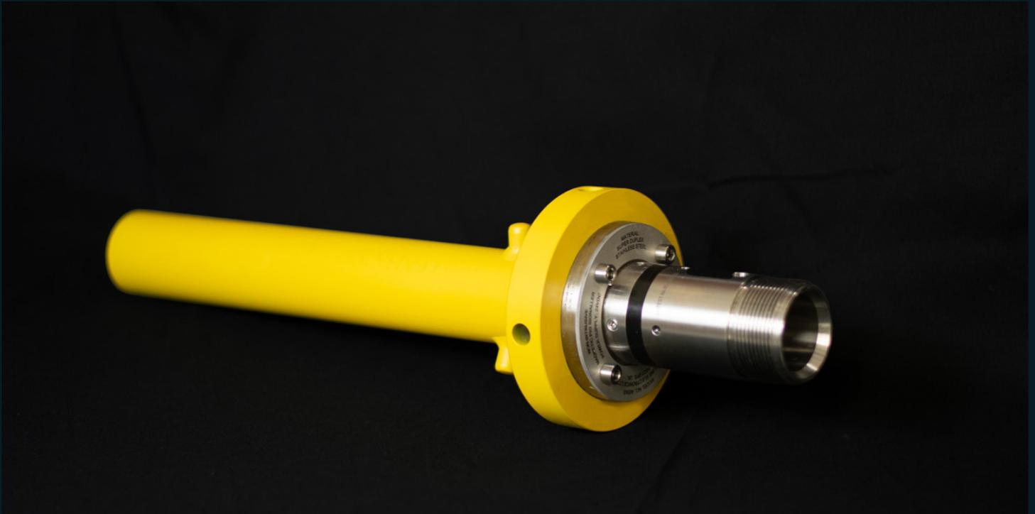
The 4004S Pig Signaller is a permanently deployable, externally powered pig signaller. The 4004S detects and signals the passage of magnetic pigs at critical points along a subsea pipeline.
