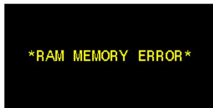
At switch ON the LOOP conducts a self-check on the RTC circuitry as per section 4.1 TURNING ON. If any problems are found then the error message shown will be displayed and the LOOP will reset all system variables to default values. Please contact IK Trax if you see this message. The most likely cause is that the coin cell has expired. See section 14.3, ROUTINE MAINTENANCE AND STORAGE, for more information.
