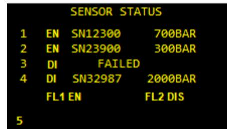
If a sensor is shown as FAILED but is connected its cable and connections should be checked.
