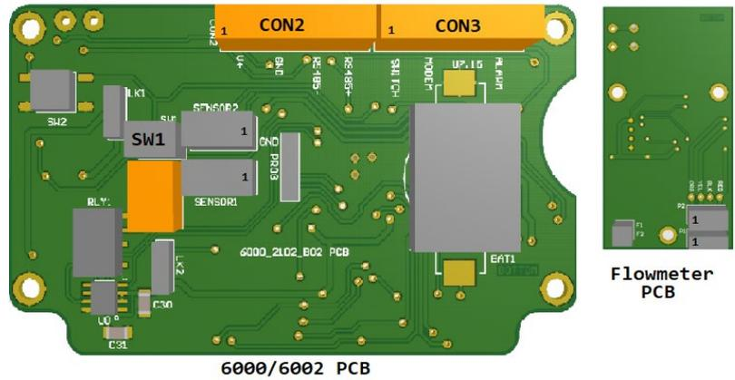
Connections are made to the internal PCBs by wires to the Burton connectors. Where a flowmeter PCB is present (fitted to the battery compartment plastic cover) the battery is connected to connector block visible on the rear of the PCB.
