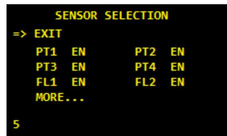
If a sensor is disabled then the LOOP does not try to communicate with the sensor. Sensor 'offline status' is logged for disabled sensors.
