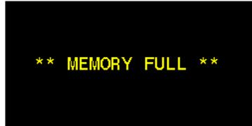
If MEMORY OVERWRITE is DISABLED and the logger memory is FULL then the logger will not log any new readings and this error message will be shown every time the logger attempts to log.
