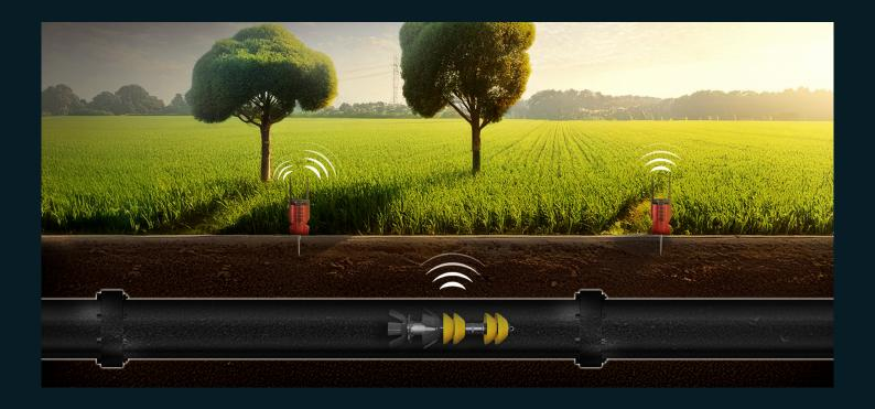
Our partner PigRun was invited to demonstrate the Patriot AGM remote tracking technology during a multi-day pigging operation on a 12 inch Enbridge gas pipeline in Kitchener, Ontario. The pipeline spanned approximately 24 kilometres and involved several cleaning runs over three days. The cleaning program included six pigs of varying types (foam, brush, magnetic) and one gauge plate, as part of a scheduled maintenance operation.
